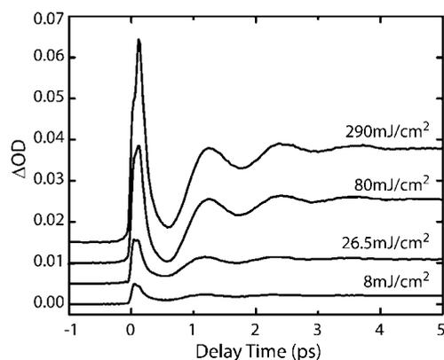
**Figure 1.** Pump/probe transient absorption data of colloidal  $\text{Fe}_3\text{O}_4$  nanocrystals obtained with 780 nm pump and 550 nm probe at various excitation fluences.
