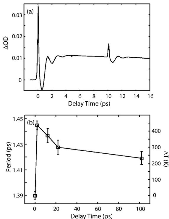
**Figure 4.** (a) Transient absorption data from the two-pump/probe measurement. (b) Time dependence of the coherent phonon period and the estimated lattice temperature obtained from the two-pump/probe measurement.
