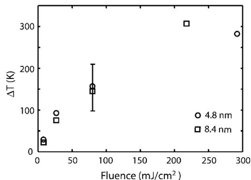
**Figure 3.** Excitation fluence dependence of the lattice temperature estimated from the period of coherent phonon. The error bar shown in the figure is a typical value.
