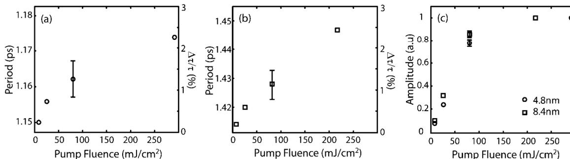
**Figure 2.** Excitation fluence dependence of coherent phonon period for 4.8 (a) and 8.4 nm (b) nanocrystals. A typical error bar is shown on each panel. On the right y-axes of panels a and b,  $\Delta\tau/\tau$  represents the fractional change of period  $[\tau(F) - \tau(0)]/\tau(0)$  described in the text. (c) Excitation fluence dependence of the amplitude of oscillation in transient absorption data. The amplitudes are normalized to the maximum value for the nanocrystals of both sizes.
